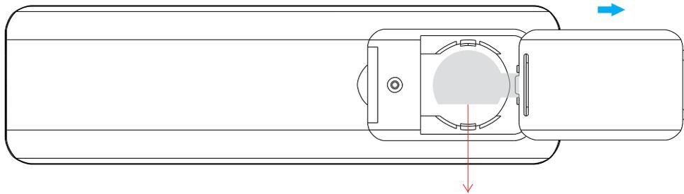
**Note:** Before the first use, please remove the protective film on the battery.
