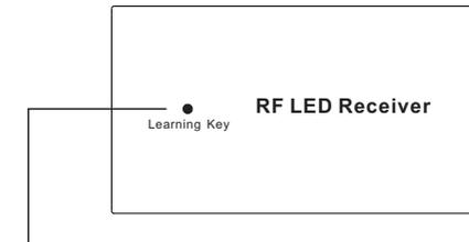
**Step 2:** Click the "Learning Key" button on RF receiver or re-power on the receiver three times continuously to set it into pairing status
